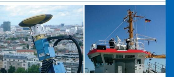
On sounding ships and dredgers, SA*POS*<sup>®</sup> has catered for a high resolution 3D data acquisition of the river beds with centimeter accuracy for many years now.
